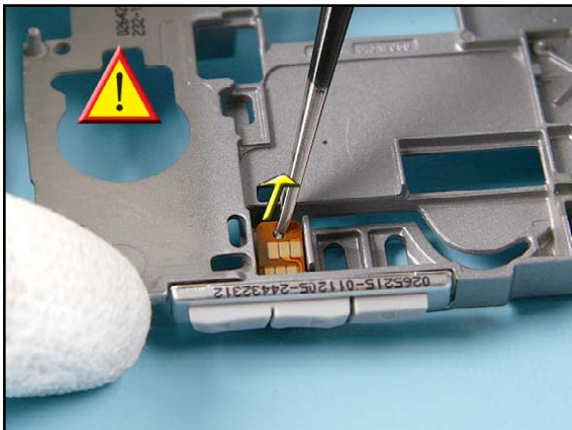
25. Unlock the SIDE BUTTON MODULE ASSY...
