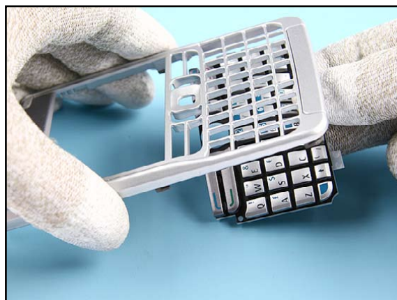
16. Separate the KEYMAT from the A-COVER ASSY.
